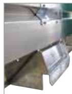
3-point hitch. Reinforced by a thick bolted plate.
