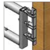
Example of mounting on 200 x 200 mm wood posts with U-turn bracket.
