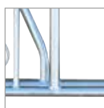
Ø 42.4 mm neck bars with guard bars welded to the double panel. Identical intervals to the neck bars initially mounted on a standard headlock. Allows a range of neck adjustments from self-service (full clearance) to neck reduction to that of young animals.
