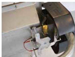
Polyresistance heating unit 24V-80W mounted in the housing.
