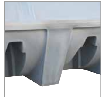
Baffles integrated in moulding, vary according to capacity, avoids liquid movement during transport. Number of baffles depends on the water tank's size.
